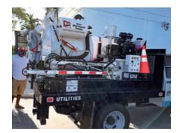
Skid system allows for simple mounting to a flatbed truck.
