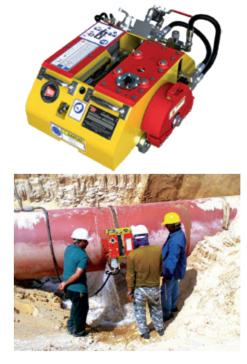
The Trav-L-Cutter can cut vertically, horizontally or anything in between
