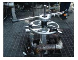
RS-2 shown with optional universal handwheel adapter on a rising stem valve
