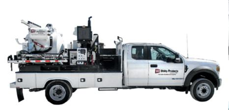
Knapheide / Wachs Valve Maintenance Truck Service Body with Integrated Wachs Service Body Valve Maintenance Skid
