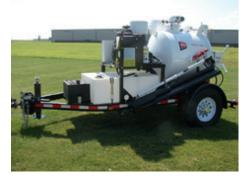
Power pack provides pressure washer system and 500CFM vacuum
